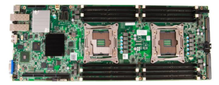
This motherboard has 2 **sockets** to plug **microprocessors**. A microprocessor is a **multicore** technology.
