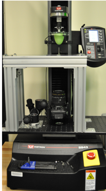
Figure 1.8: The final Instron set-up that enables imaging.
