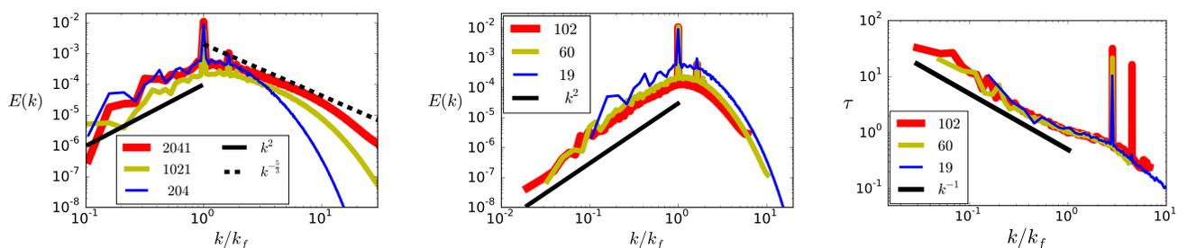
(Left) Energy spectrum for different Reynolds numbers. (Center) Energy spectrum for different scale separations at fixed  $\nu/k_f$ . (Right) Correlation time for different scale separations at fixed  $\nu/k_f$ .
