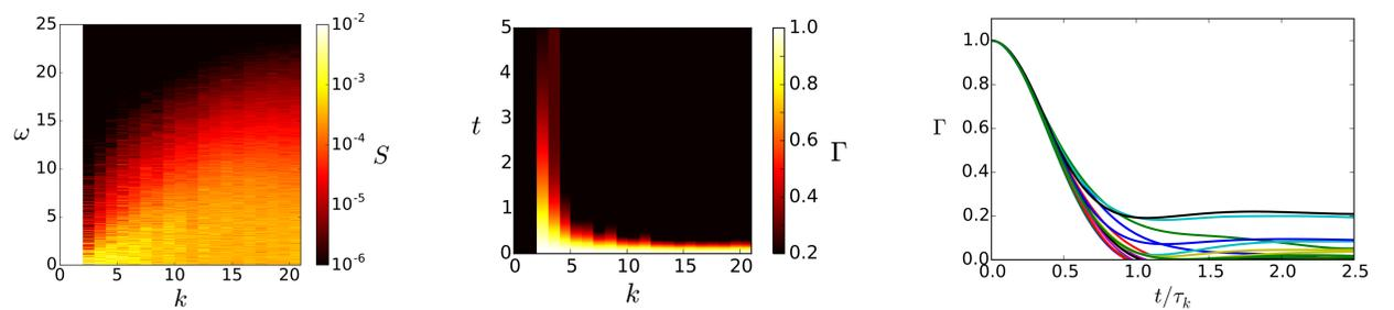
(Left) Power spectrum  $S(k, \omega)$ , (Center) normalized correlation function  $\Gamma(k, t)$ , (Right) re-scaled correlation function  $\Gamma(k, t/\tau_k)$  of the modes of Taylor-Green symmetric absolute equilibrium.
