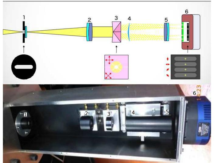
**Figure 2.** Scheme and photography of the ToPo instrument. 1: Field stop followed by the field lens. 2: Collimator lens. 3: Wedged double Wollaston. 4 and 5: Camera optics. 6: QSI632 CCD camera
