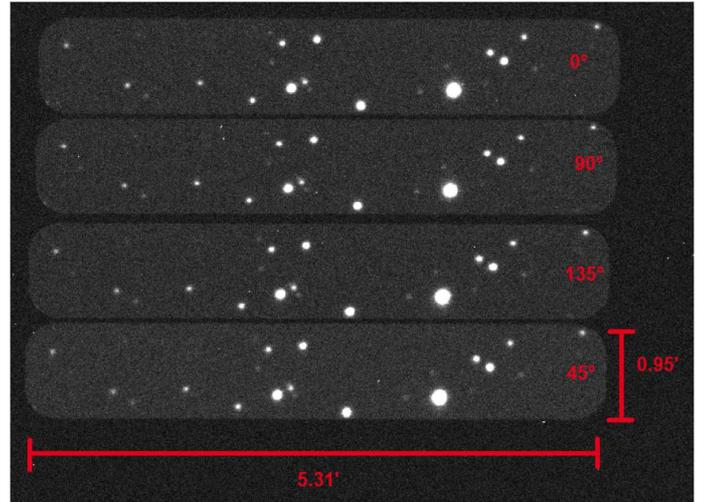
**Figure 1.** Example of a ToPol frame. The four strips correspond to the four images of the field of view of ToPol. Each strip corresponds to one specific polarization state (respectively from top to bottom 0°, 90°, 135° and 45°).
