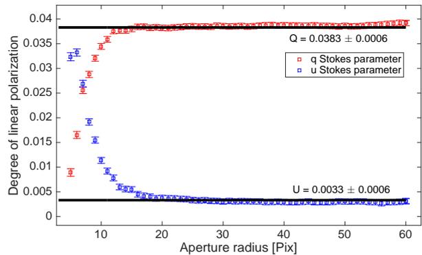
**Figure 3.** Example of a typical curve of growth. The red squares represent the  $q$  reduced Stokes parameter as a function of the aperture radius (in pixels). The blue ones correspond to the  $u$  reduced Stokes parameters. The black lines represent the best value of  $q$  and  $u$ . The  $u$  curve was reversed for display reasons.
