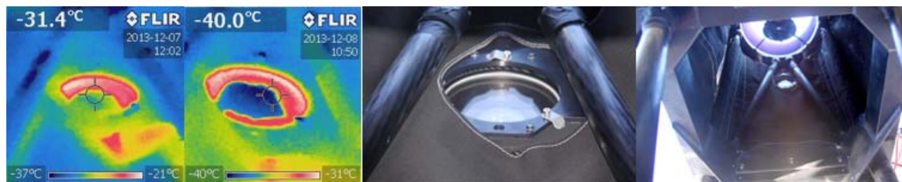
Fig. 13 Photographs of the camera entrance window in the infrared and visible. First photograph from the left: Camera box entrance window in the IR when heated to +10 °C inside the camera box. Second photograph: Camera window in the IR when heated −8 °C (2nd IR image). Third photograph: Blowup of the camera window in the visible to scale with the IR photographs. Fourth photograph: Visible photograph is taken from near the M1 mirror, looking up towards the camera window and the M2 mirror.
