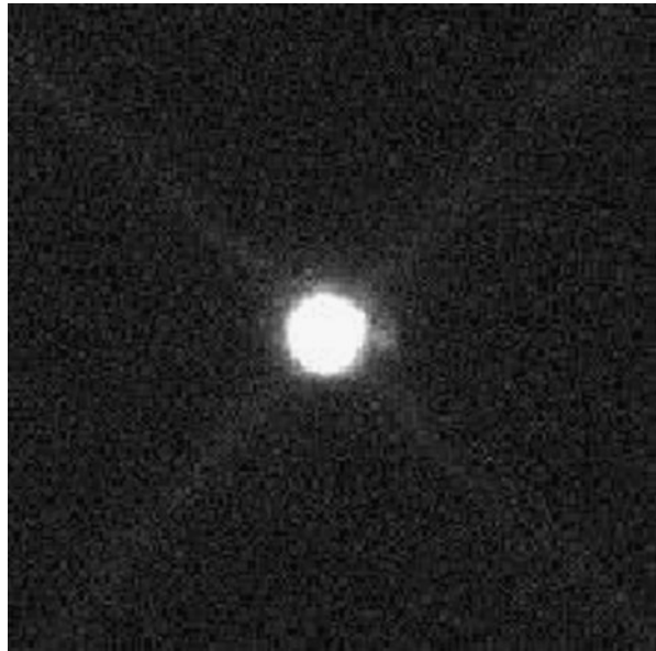
Fig. 5 Image of the double star STF 2726 (52 – Cyg) obtained with the Generation 1.5.1 prototype (115 mm effective aperture). The companion on the right hand side is 4.5 magnitudes fainter than the central star , and separated by 6.4''
