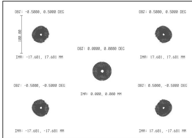
Figure 3 : Spot diagrams for different fields in the science path
