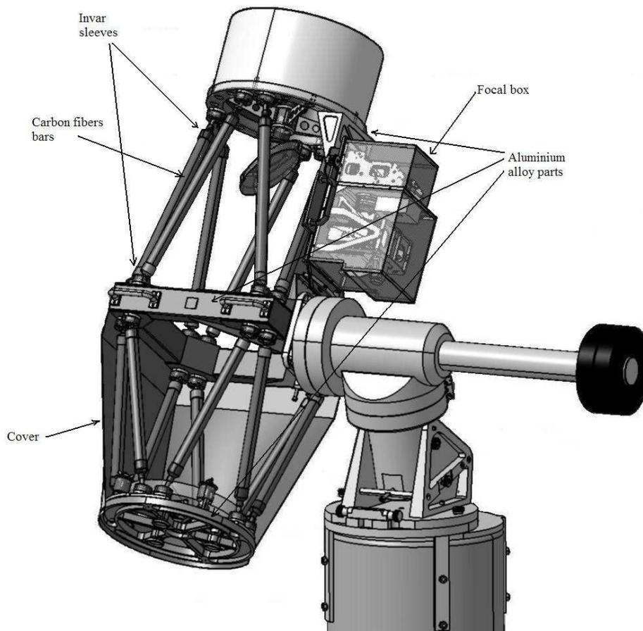
Figure 5 : Mechanical structure of the telescope
