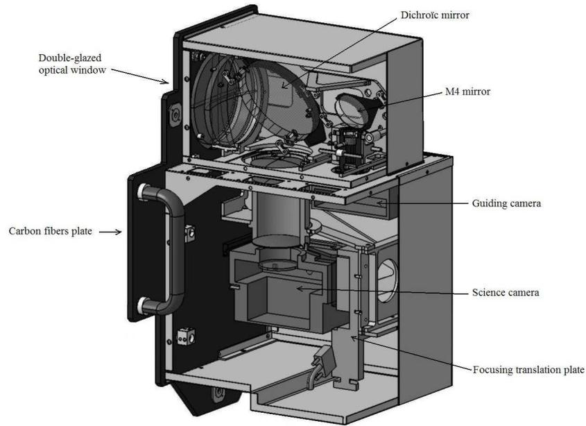
Figure 6 : Design of the focal box (cutaway view)
