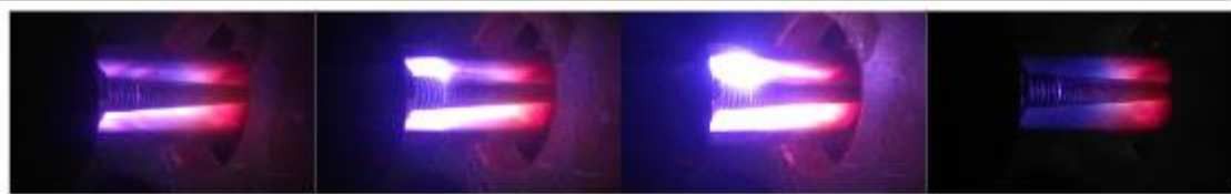
Plasma to excite He to metastable state : 20 eV, 2h.
