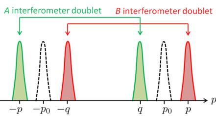
The A doublet and the B doublet do not have the same Bragg transition resonance frequency
