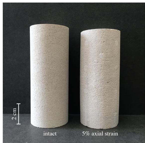
**Figure 1.** Photograph of an intact sample and a sample deformed up to 5% axial strain at  $P_{\text{eff}} = 50 \text{ MPa}$ .
