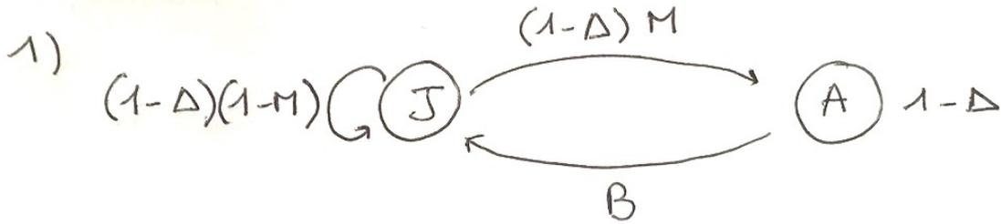
the system can be described by the matrix:  $C = \begin{pmatrix} (1-M)(1-\Delta) & B \\ (1-\Delta)M & 1-\Delta \end{pmatrix}$
