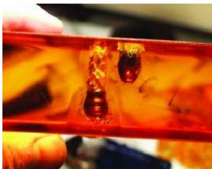
**A 1.5-inch-thick polydicyclopentadiene resin prepared with ruthenium technology is impenetrable to 9-mm bullets.**
