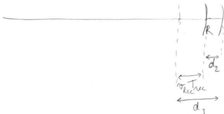
$$d_3 = c T_{rec} = v_{rec} T_{rec} + (c - v_{em}) T_{em}$$
