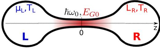
FIG. 1. Two reservoirs (L, R) can exchange particles through a smoothly tapered constriction inside which the spatially dependent and attractive gate potential  $E_G$  is varied.
